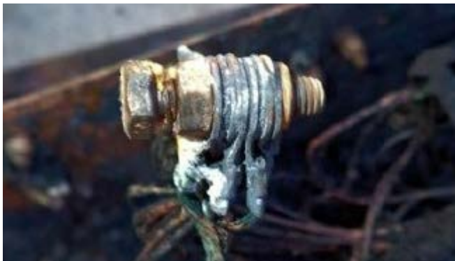
Multiple ring terminals on a single stud can result in a hot terminal developing. Photos: Peter Hart/Hartwood Consulting
