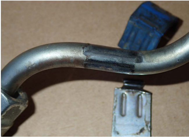
Fuel leaks from injector tubes should never be ignored. Above and below: Sections of high-pressure fuel line. The green arrow indicates where fuel would leak from. Photos: Peter Hart/Hartwood Consulting
