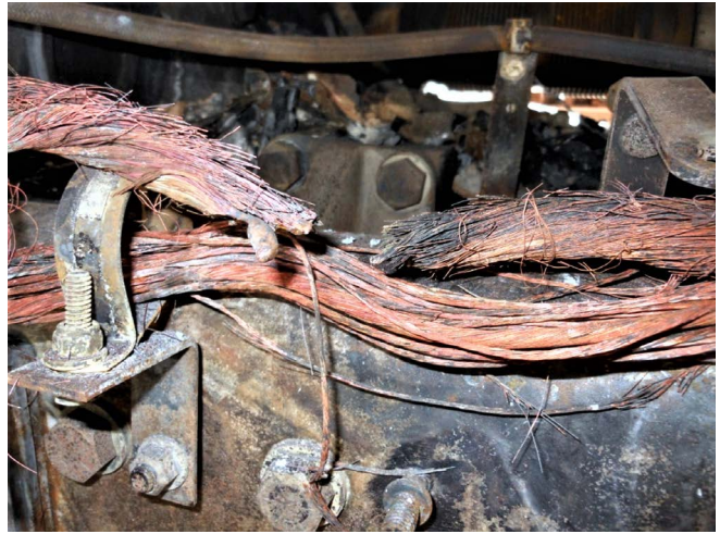
A main cable rub at a metal-spined clamp. Photo: Peter Hart/Hartwood Consulting
