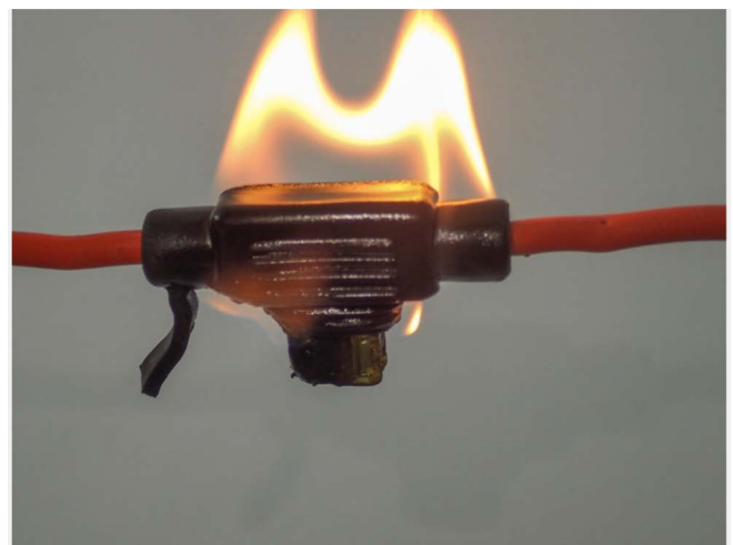
Some electrical components burn freely, which is a problem. Notice that the cable insulation does not burn freely. Photo: Peter Hart/Hartwood Consulting
