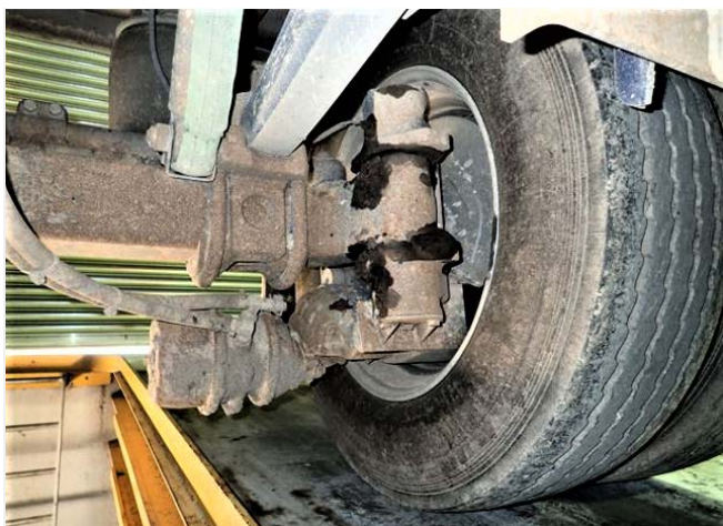
Look for road-strike damage to brake actuators. Photo: Peter Hart/Hartwood Consulting
