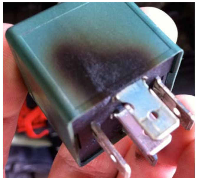
Pyrolysis of a polymer relay case indicating high and unacceptable operating temperature. Photo: Peter Hart/Hartwood Consulting
