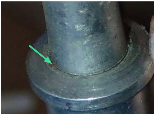
Fuel leaks from injector tubes should never be ignored. Above and below: Sections of high-pressure fuel line. The green arrow indicates where fuel would leak from. Photos: Peter Hart/Hartwood Consulting
